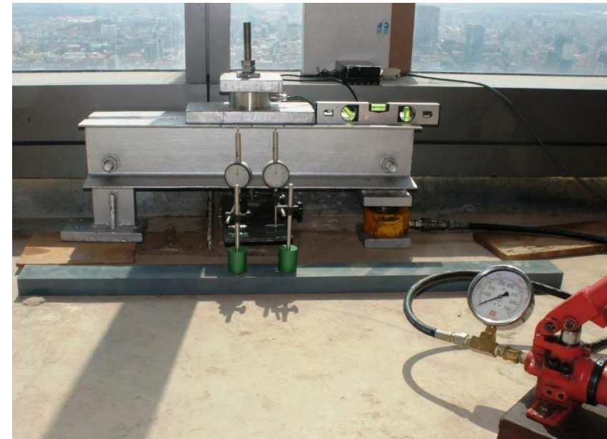
Pull-out test setup as per ASTM E488
